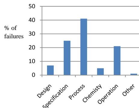
Figure 2: Major Causes of Coating Failures [13]
